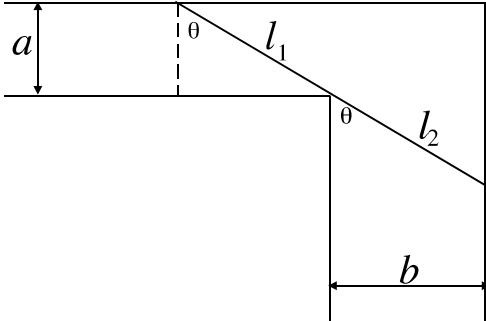
With  $\theta$  as shown, the length  $l$  of the line is given by  $l = l_1 + l_2 = \frac{a}{\cos \theta} + \frac{b}{\sin \theta}$
